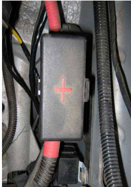
Gambar 16.6. Junction Block dan relay block
