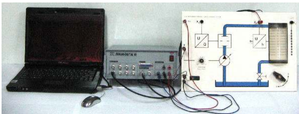
Gambar 9.47 Rangkaian Percobaan Water Level Control
