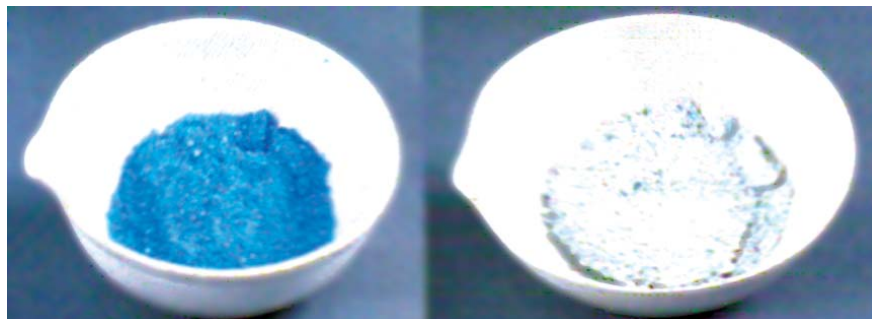
Gambar 3.11 \text{CuSO}_4 \cdot 5 \text{H}_2\text{O} (kiri) dan \text{CuSO}_4 (kanan). Sumber: Chemistry, The Molecular Nature of Matter & Change, Martin S. Silberberg, 2000.
