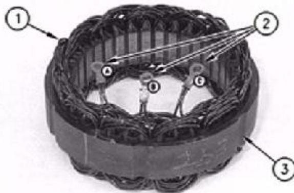
Gambar 4.40 – (1) Stator, (2) Stator Lead, (3) Stator Frame
