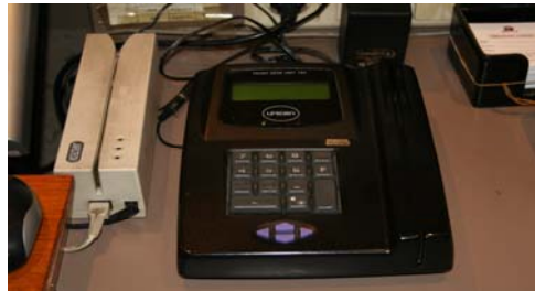
Gambar 3.16. Key encoder machine
