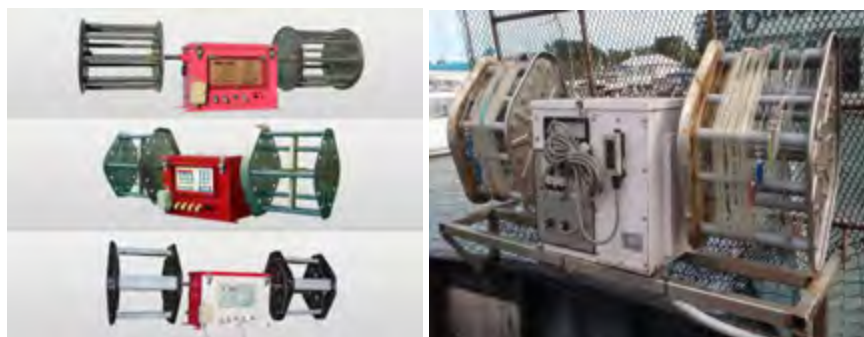
Gambar 166. Mesin pancing cumi otomatis (jigging automatic machine)
