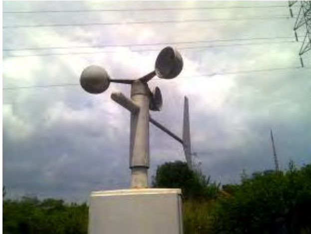
Gambar 88. Anemometer tiga mangkok
