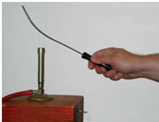
Sumber: www.physics.upenn.edu Gambar 4.6 Saat dipanaskan, bimetal melengkung.
