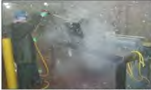
Figure 1. When used as a cleaning tool, high pressure water should be applied in a controlled manner to avoid generating aerosols that can migrate from non-product contact surfaces to clean product contact surfaces.
