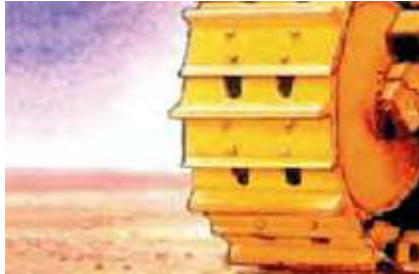
Gambar 13.12 Tipe Single grouser shoe
