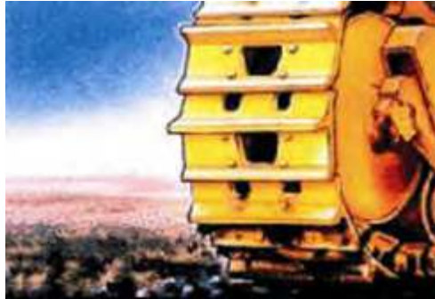
Gambar 13.16 Trapezoidal Center Hole Shoe
