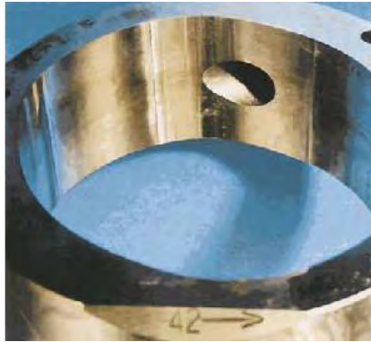
Gambar 4.37 Penampang cam ring (wear)
