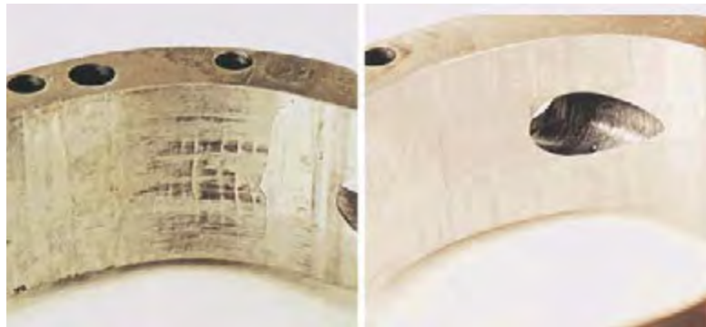
Gambar 4.40 Penampang cam ring (aerated, frosting and ripple)
