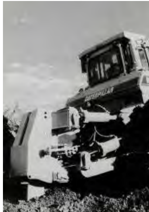
Gambar 6.3 Operasi dozer saat ripping
