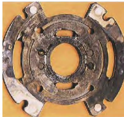
Gambar 4.35 Penampang flex plate (burn oil residu)
