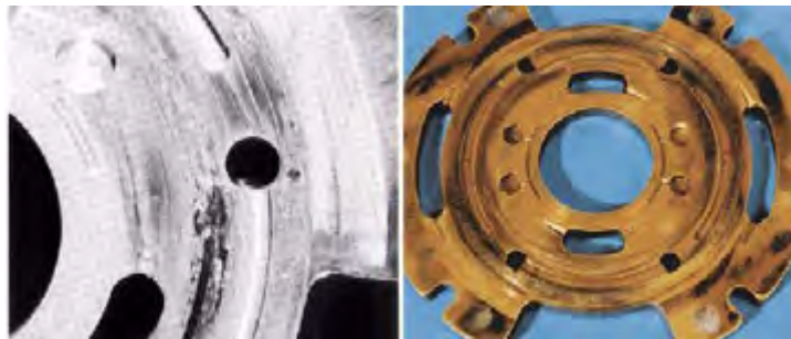
Gambar 4.30 Penampang flex plate (scratches)
