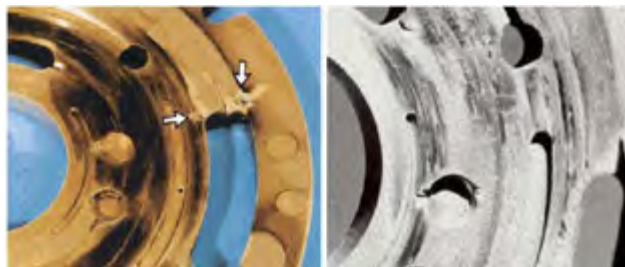
Gambar 4.31 Penampang flex plate (erotion)
