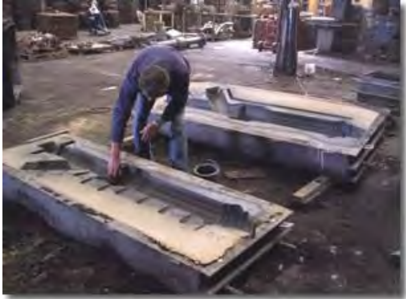
Mould for castiron ventcolum being prepared for casting
